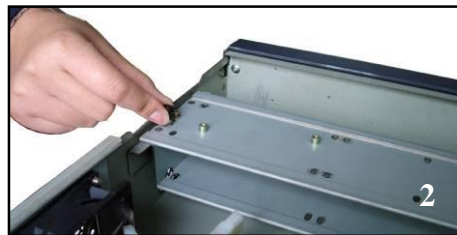
2. Remove the HDD bracket from internal unit
