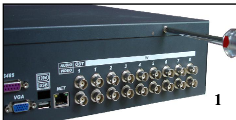
1. Remove the upper cover of the DVR
