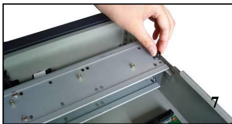
7. Fix the HDD bracket into the internal unit
