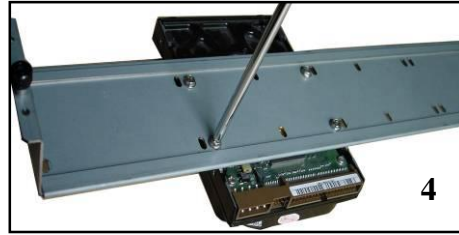
4. Install the HDD. Note the HDD is placed upside down. Please make sure bracket is in correct position.
