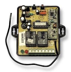
Setting up the correct mode for the receiver - The receiver has 4 different operating modes these being, Mimic, Delay, Toggle and Latch. You need to decide what mode you want for your particular application.
