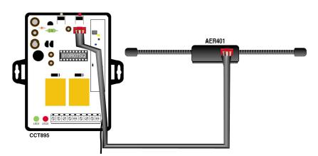
The maximum output power of the key fob is fixed so the only way to extend the range the two devices working together is to make the receiver more sensitive. To do this you can add an external dipole aerial (code AER401). This can extend the range up to about 300m in *ideal conditions*. Please remember solid obstacles will attenuate the key fobs signal and reduce the range. Ideal conditions are direct line of sight with no obstacles in-between
