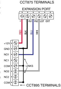
The second button can be used to control external lighting if you have a flood light controller connected to the CCT875.
