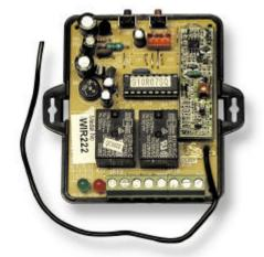
**Setting up the correct mode for the receiver** - The receiver has 4 different operating modes these being, Mimic, Delay, Toggle and Latch. You need to decide what mode you want for your particular application. NOTE - If you are using the receiver with the Advanced Vision CCT875 panel you need to leave the receiver in its factory default "Mimic Mode"
