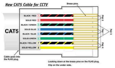
go to the end of the plug or they won't all be crimped!! You need to put an RJ45 plug using the same colour coding on both ends of the CAT5 cable, ensuring that each colour goes to the correct pin in the plug.
