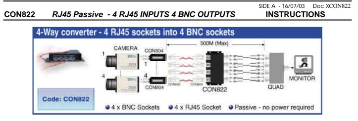
It is possible to send video signals down one CAT5 cable. The CON822 is a useful balun for terminating 4 separate CAT5 radials from balun types CON804 or CON805 in to one 4-way balun.
