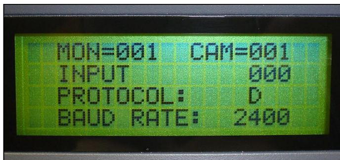
LCD of keypad CCT786 & CCT768 with correct default setting for this PTZ at address 1
